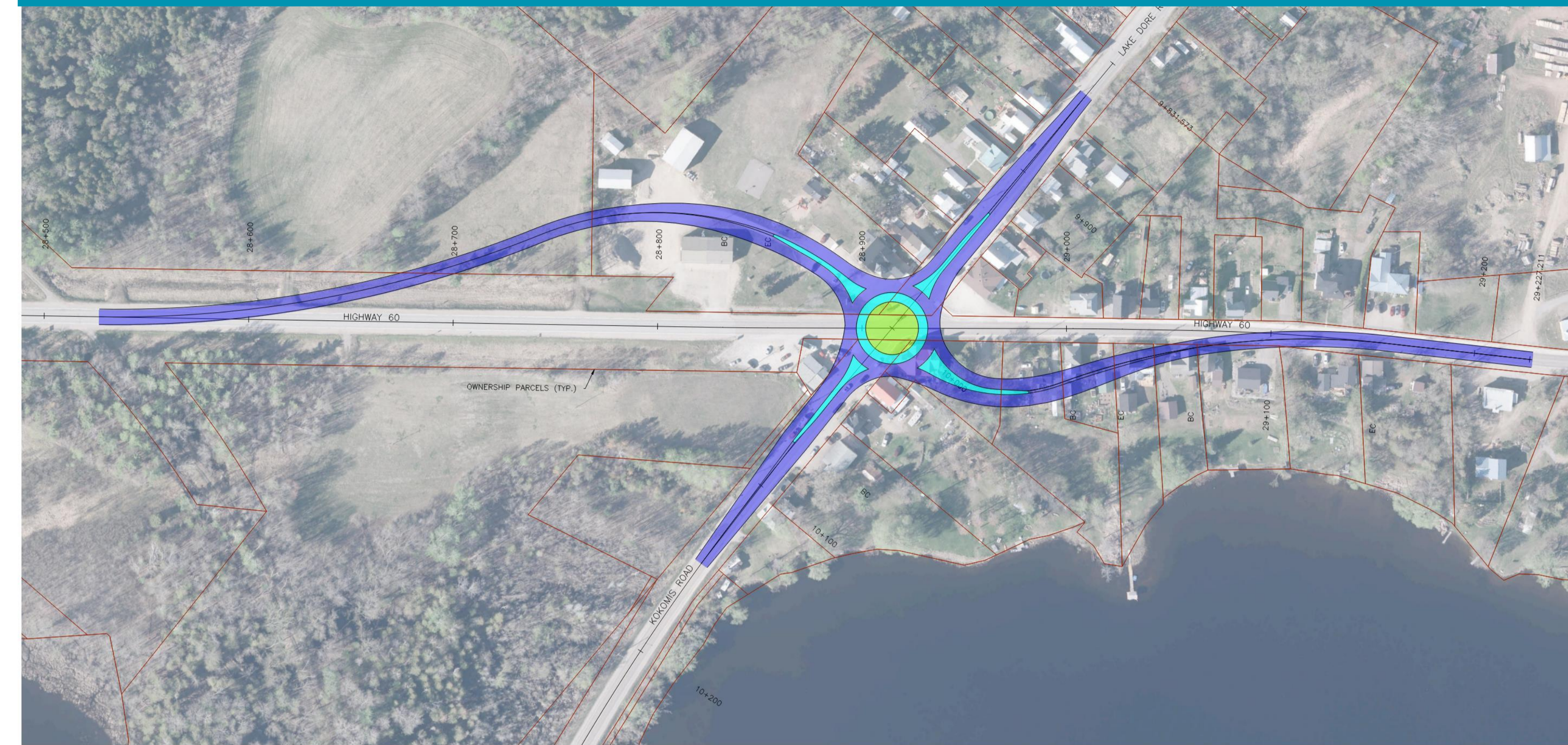
Roundabout skewed for improved approach angles
